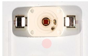
Status of LED: no degradation
